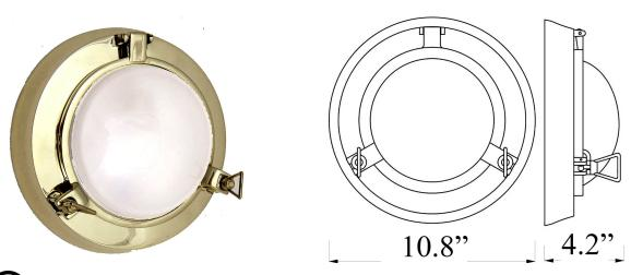
UL Listed; Dry Residential & Commercial Use <u>Max Wattage:</u> 100w LED Equivalent; 75w Wall, 60w Ceiling Incandescent Bulb ; Medium Base (E26) Socket, Dimmable (GU-24 also available) <u>Glass:</u> Frosted Glass Only <u>Mounting:</u> 10.8" Mounting Surface, attaches to standard box. All Installation Hardware Provided
